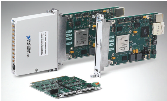
Fig. 2 The FlexRIO series FPGA modules use external adapter modules for I/O customization and are available in both PXI and PXI Express versions.
